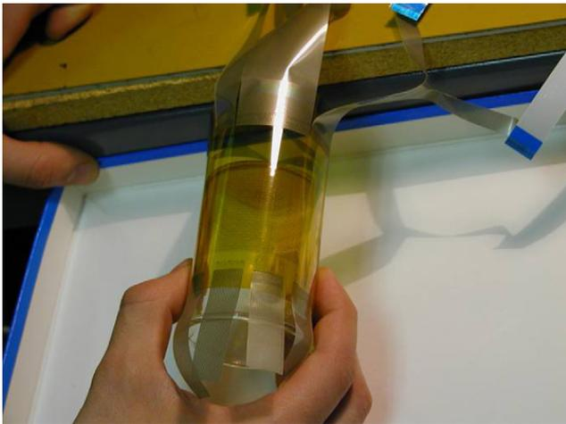
Fig. 15. The sample is strained around a glass beaker to maintain a constant radius of curvature.
